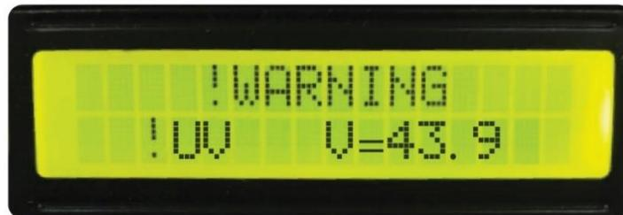
This means the module voltage has decreased below the cut off value of 44V. The LCD shows the voltage at that time as well (in the illustration, the LCD shows that the module voltage has decreased to 43.9V).
