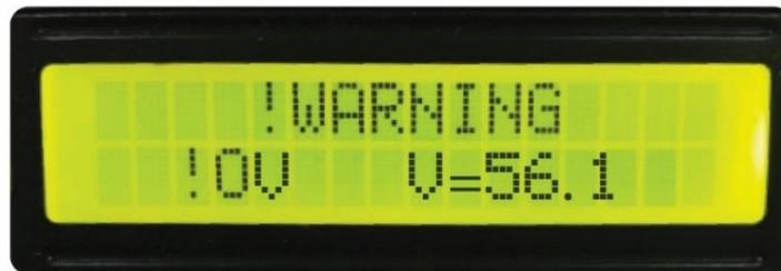
This means the module voltage has increased beyond the cut off limit of 54.5V. The LCD shows the voltage at that time as well (in the illustration, the LCD shows that the module voltage has increased to 56.1V).
