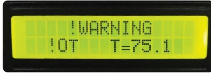
This means that the temperature of the module has increased beyond the cut off value of 75°C. The LCD shows the temperature at that time as well (in the illustration, the LCD shows that the module temperature has increased to 75.1°C).
