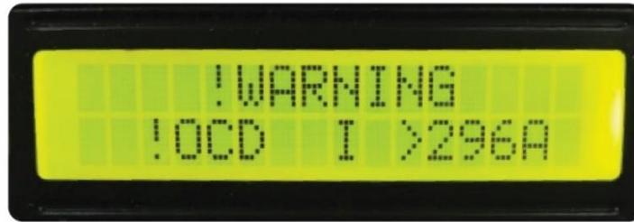
This means the current has increased beyond the cut off current of 296A (in the illustration, the LCD shows that the module current has increased above 296A).
